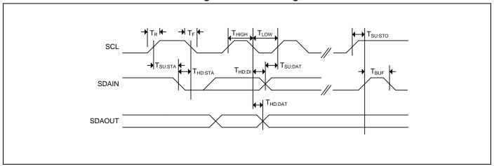
Figure 5.7. Write Cycle Timing
